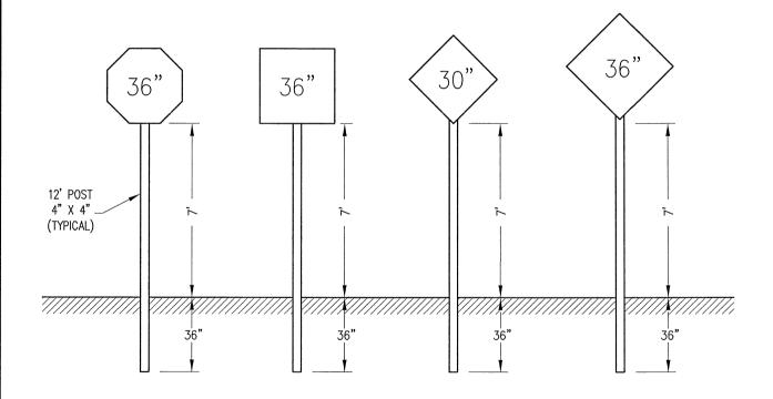
NOTE: USE THIS DETAIL WHERE ANY PORTION OF SIGN EXTENDS OVER ANY PAVED ROADWAY SURFACE, SIDEWALK OR WALKWAY.
