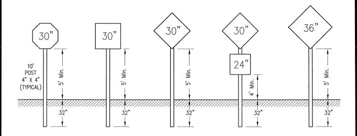
NOTE: USE THIS DETAIL WHERE ANY PORTION OF SIGN DOES NOT EXTEND OVER ANY PAVED ROADWAY SURFACE, SIDEWALK OR WALKWAY.
